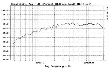
Driver is mounted rigidly in free air with no baffle or enclosure. Input signal is a stepped sinusoidal at 1VRMS. Impedance is measured using constant-voltage method. No smoothing 2.83VRMS and normalized to 1m. 1/12 octave smoothing was applied. was applied.
