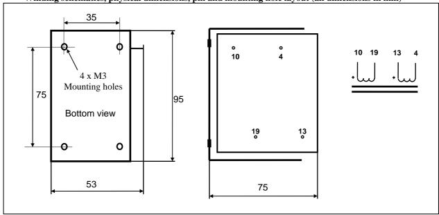
Weight:1.35 kgStatic resistance of each winding: $1.7 \Omega$ Max current through each winding (10W heat dissipation):1.7 AIsolation between windings / between windings and core:4 kV / 2 kV
