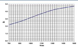
Power Compression Losses were calculated after 2 hours period applying a pink noise signal filtered between 25 and 200 Hz.
