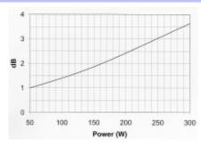
Note: These losses are calculated from a five minutes AES power test applying band limited pink noise (25-1200 Hz). The loudspeaker is free-air standing.
