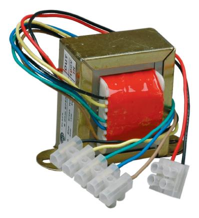
The Apart T60 is an 8 Ohm to 100 Volts transformer. By using the T60 you can change a standard 8 ohm loudspeaker into a 100 Volts loudspeaker.
