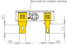
Thickness, both terminals: 0.5 mm Terminal plating: Gold
