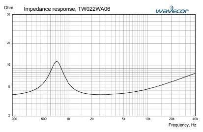
Measuring conditions, impedance Driver mounting: Free air, no baffle, back side open (no cabinet) Input signal: Semi-current-drive, nominal current 2 mA Smoothing: None
