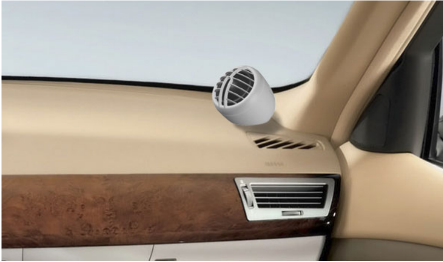
Wavecor's 30mm car tweeter angle mounted
