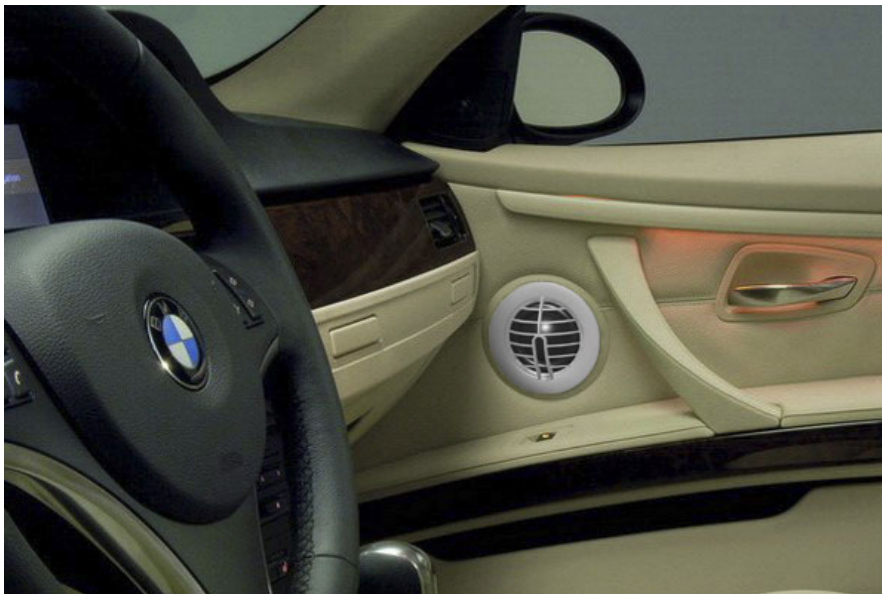
Wavecör's 30mm car tweeter flush mounted
